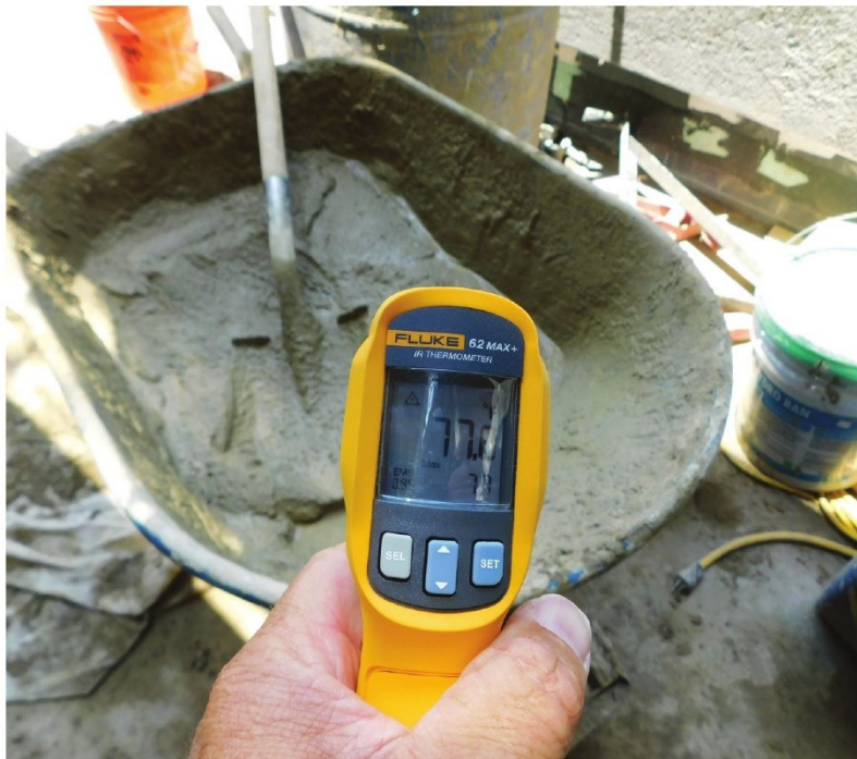
A laser thermometer can be used to document the temperature of the substrate or materials not exceeding 32 C (90 F).
