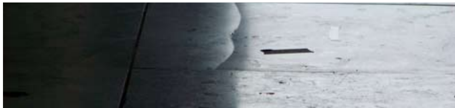
Indent fractures are not easy to see; typically they can only be seen from an angle when light reflects off them.
