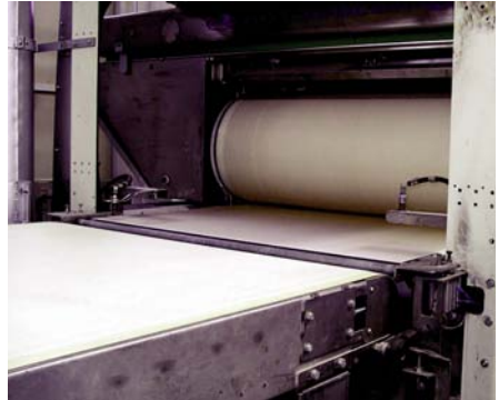
A roller press early in the production stage of Kale's oversized flexible porcelain Kalesinterflex slabs that have a thickness of only 3 mm.
